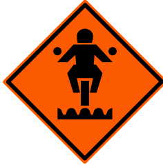
Sign warning motorcyclists of a rough or uneven surface.
